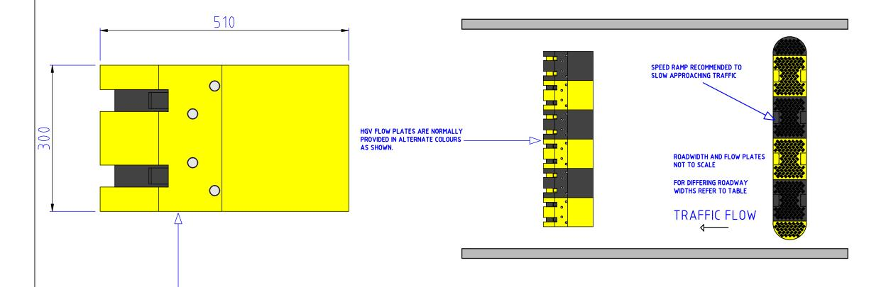
TRAFFIC FLOW CONTROL PLATES ARE DESIGNED TO ENCOURAGE ONE WAY TRAFFIC FLOW AND PREVENT UNAUTHORISED ENTRY/EXIT WITHIN ANY LOCATION.
